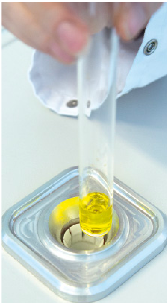
Close-up of a sample tube Toebes is placing in the NMR machine.
